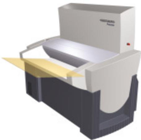
Once on the plate table, each plate is automatically recognized and centered.
